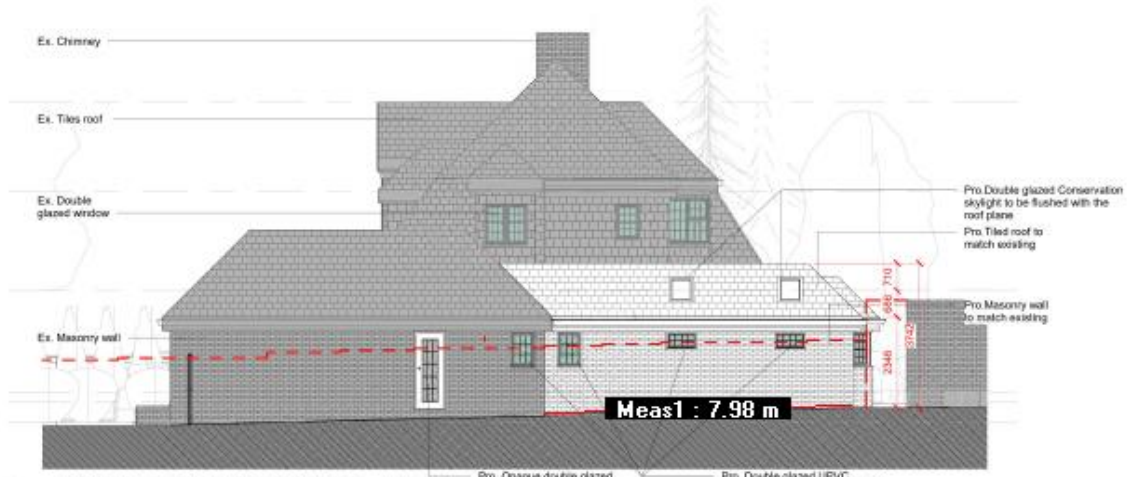
1 Proposed Elevation - East 1 : 100
